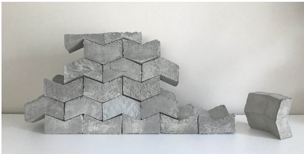
Figure 10 A sample wall made by V-INCA bricks
