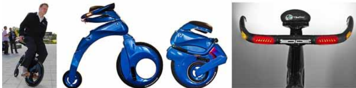
Figure 13. from left: The Yike Bike in use, unfolded and folded. The handle bars wrap around behind the rider and accommodate headlamps at the front and break lights and indicators at the back. [Yike Bike.]
