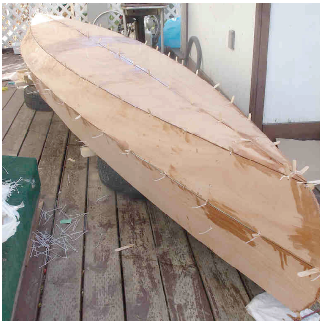
Figure 1: A stitch and glue canoe in production. Photo: Kevin Saff
