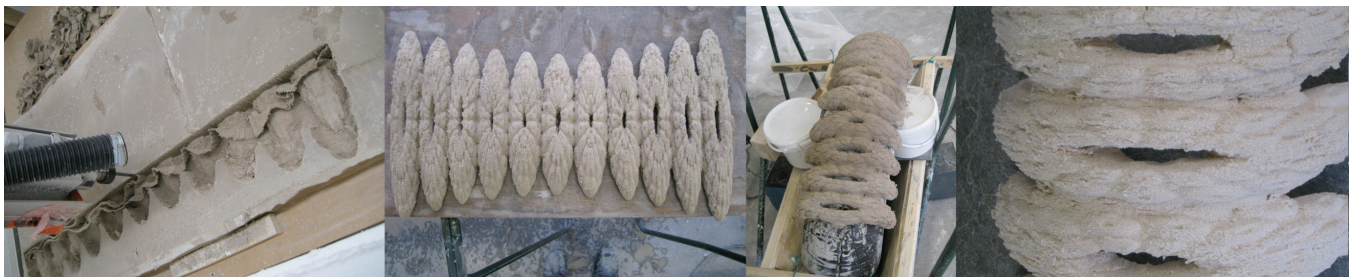
Figure 5: Machining hardened sponge, completed part soaked in clay slip, part placed over rounded primary form for drying, fired part showing excellent detail
