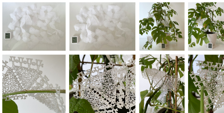
Figure 9. Structures without water (42% of humidity) and with sprayed water (55% of humidity); structures arranged around a plant without water (42% of humidity) and with sprayed water (63% of humidity); structures arranged around a plant and close-ups.
