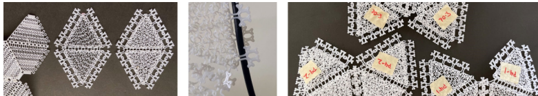
Figure 8. Different joint types and sizes; test for the grip-ability to the plant's stem, structures with different meshes. The one that performed better and was chosen for the final structure was the P4-1.
