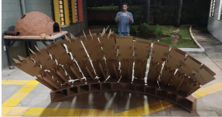
Figure 6. 1:1 Scale assembly test. Source: Author, 2023.
