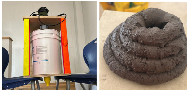
Figure 6. Second prototype of the extruder and extrusion results.
