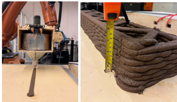
Figure 8. Fourth prototype of the extruder and extrusion results.
