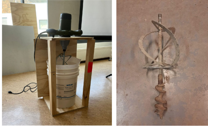
Figure 5. First prototype of the extruder and the mixed with the screw.
