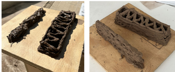
Figure 4. Initial tests of the paste consistency, conducted manually.
