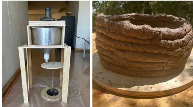
Figure 7. Third prototype of the extruder and extrusion results. On the left, a turntable to simulate the printing process before mounting the extruder to the robot.
