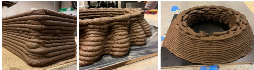
Figure 10. Final printing experiments using a wall design, a ribbed dome and a double layer dome.
