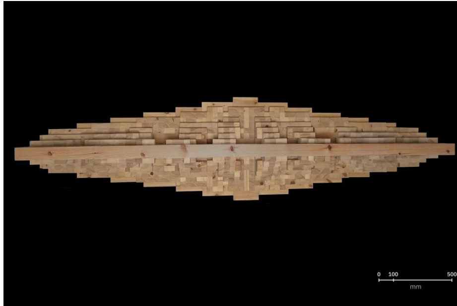
Figure 7. Bottom view of the Re-VoxLam Truss. Voxel density aggregations and lamination techniques are used to realise the complex 3D geometry.
