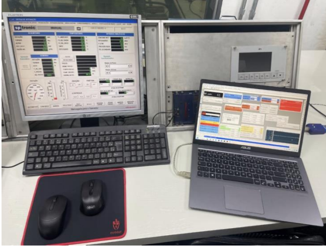
Figure 5: E_CAT software used to control the dynamometer, and INCA software used to control the engine. Both are also used for data acquisition.
