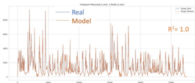
Figure 11- Model vs. Measured- CO 2 along the Cold Start
