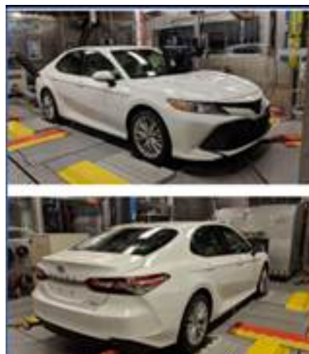
Figure 5- Vehicle on chassis dynamometer test [12]
