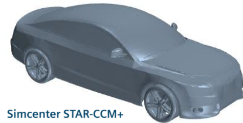
Figure 3 – EV geometry used for mesh generation.
