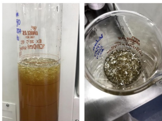
Figure 2. PC SOY100 formulation after addition of 5% synthetic ester. Partial improvement in dispersion was observed, but the mixture remained visibly heterogeneous.
