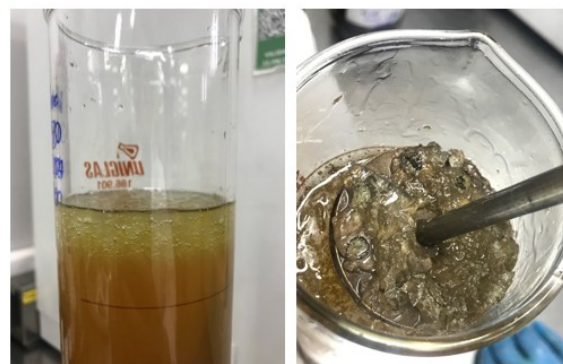
Figure 3. PC SOY100 formulation with 20% synthetic ester. Despite the higher ester content, full homogenization was not achieved, suggesting limited compatibility between the soybean oil and the ester under the tested conditions.
