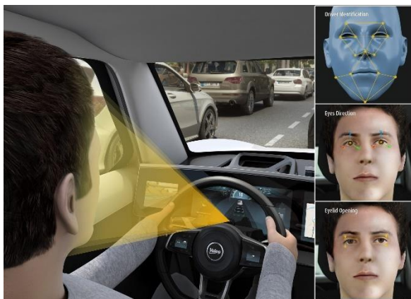
Figure 1: System for Monitoring Driver Drowsiness Signals. Available: https://www.valeo.com/en/driver-monitoring/ . Source [12].
