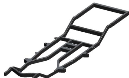
Figure 8: Simplified generic chassis Source: Nabin Mishra [5]
