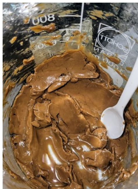
Figure 3 – Visual appearance of the rGO/Spindle sample after completion of the centrifugation washing process.
