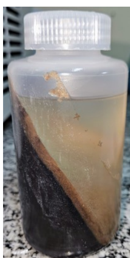
Figure 2 – rGO/Spindle 60 sample immediately after completion of centrifugation.
