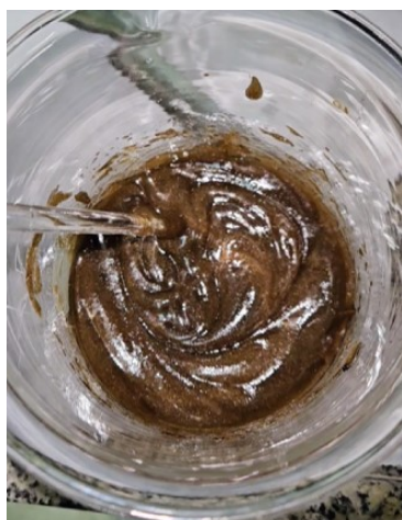
Figure 1 – Homogenization of the rGO/Spindle 60 dispersion after 15 minutes of magnetic stirring.
