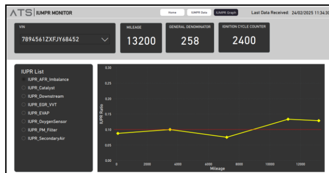
Figure 8. Dashboard with the evolution of IUMPR performance data throughout the useful life of the vehicle
