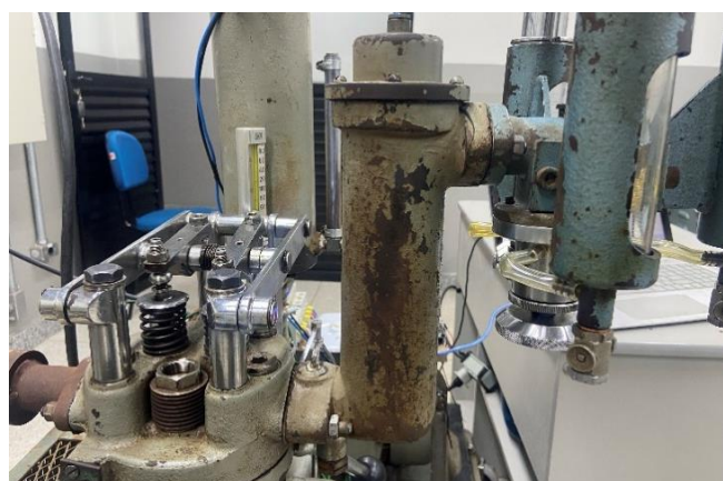
Figure 7. Heating system with electric resistance.
