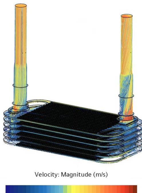
Figure 10. Streamlines (detailed model).
