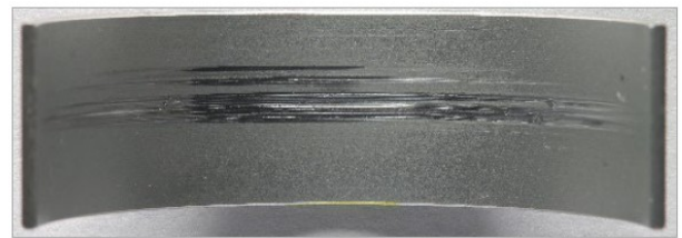
Figure 14: Development alloy+'B' after particle tolerance testing (2100 µm size particle)
