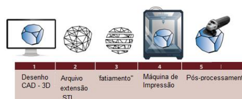
Figure 1. Manufacturing steps in AM
