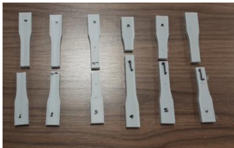
Figure 6. Specimens after tensile test, according to ASTM D638-14 Type I standard
