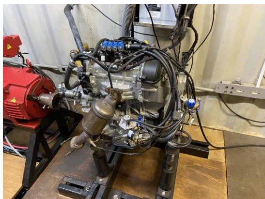
Figure 2 – Volkswagen EA211 1.0 MPI engine on the test bench
