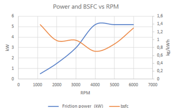
Figure 3 – Graph of friction power and bsfc by engine speeds operating without load
