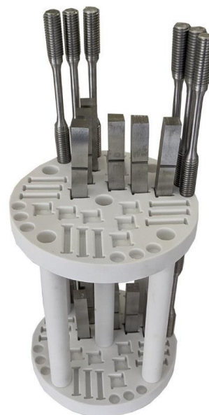
Figure 3. Alumina supports for positioning the specimens in the autoclave
