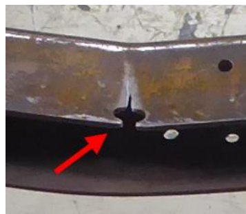
Figure 21. Broken hole after bending
