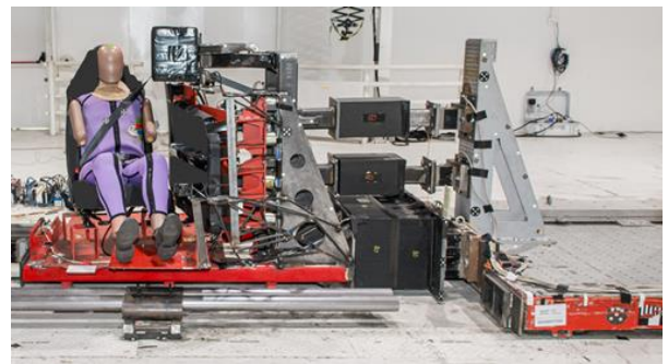
Figure 12. Sub system lateral Pole Sled test setup
