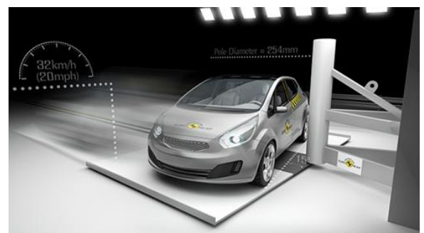
Figure 1. Euro NCAP Side Pole Impact crash test [3]
