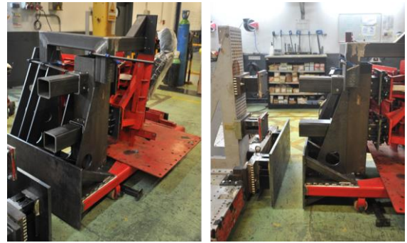
Figure 11. Construction of the sled and articulated structures
