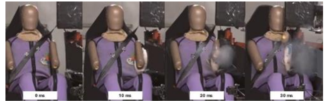
Figure 15. Dummy kinematics in physical test
