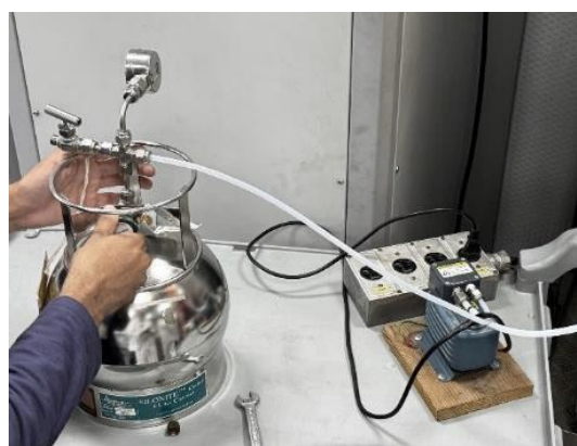
Figure 3. Sample transfer process for the steel spheres.
