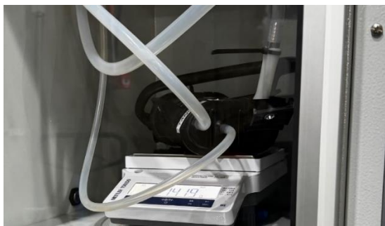
Figure 1. Vehicle vapor canister in the conditioning system during the saturation procedure.
