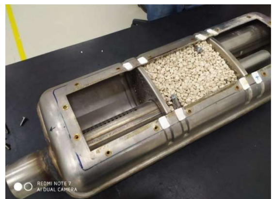
Figure 8. Reactor filled in one chamber
