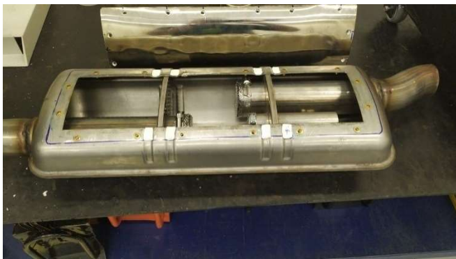
Figure 5. Designed encapsulator (reactor)
