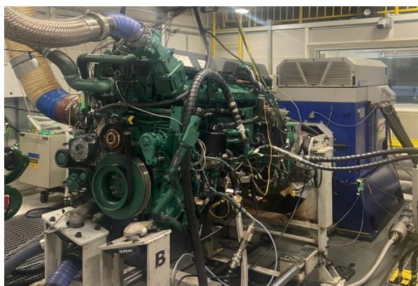
Figure 1 - Volvo EURO VI engine rigged at the test cell.
