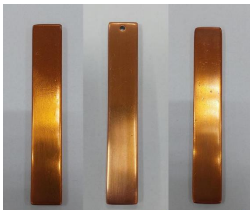
Figure 4. Copper strips after 150°C, 24 h, copper corrosion test. Left to right: DEXRON IIIH, DEXRON VI and DEXRON VI hybrid product.
