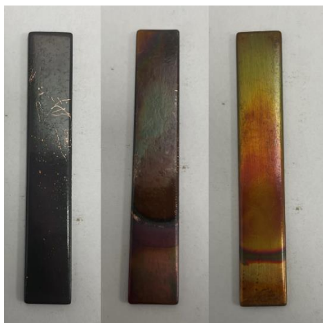
Figure 7. Copper strips after 175°C, 24 h, copper corrosion test. Left to right: DEXRON IIIH, DEXRON VI and DEXRON VI hybrid product.
