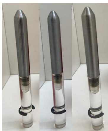
Figure 3. The 3 steel test rods after the 48 h test. Left to right: DEXRON IIIH, DEXRON VI and DEXRON VI hybrid product.
