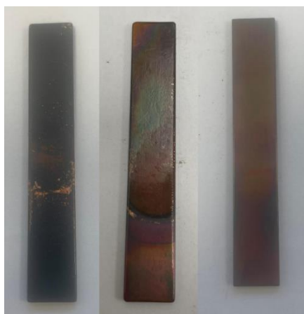
Figure 8. Copper strips after 175°C, 48 h, copper corrosion test. Left to right: DEXRON IIIH, DEXRON VI and DEXRON VI hybrid product.
