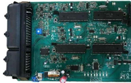
Figure 6. ECU fitted with four PIC MCUs
