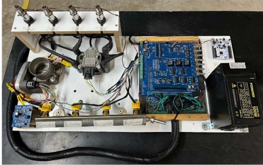
Figure 1. The full HIL setup (with actuators).
