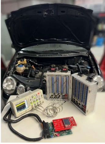
Figure 8. Final setup connecting the ECU to the real vehicle.
