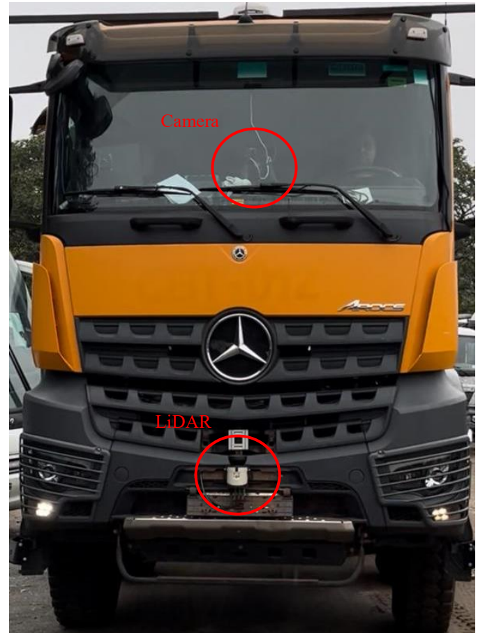
Figure 3: Front view of AROCS showing the position of the LiDAR and Camera sensors.
