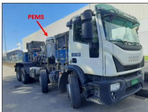
Figure 16. Vehicle, used for RDE test
