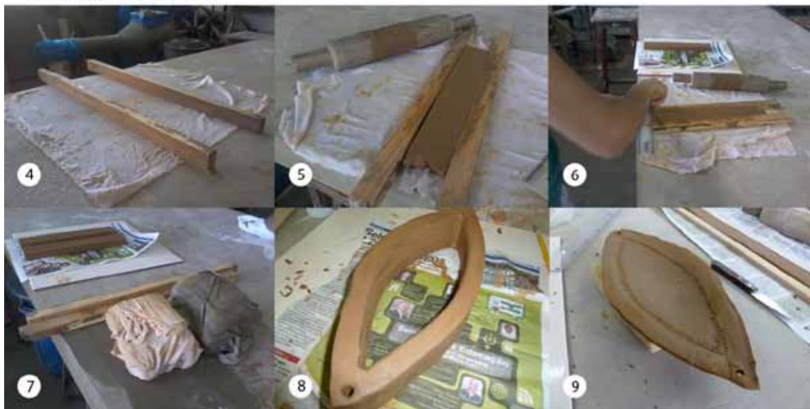
Figure 3. Detailed summary of the prototype manufacturing. Starting from the top, left to right: 1. plaster former plate; 2. clay material is placed into the former plate; 3. width and surface is brushed up; 4. Wooden boards for the equal thick plates manufacturing; 5. Plates production; 6. width and surface brush up; 7. ready plates and lid production; 8. Joining the two plates resulting in an unfinished single piece; 9. Lid shaped cut plate.
